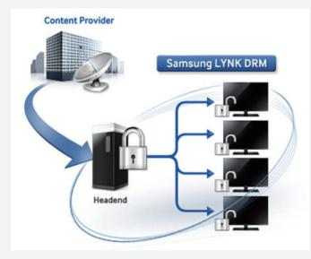
Figure 5. Samsung LYNK DRM technology allows encrypted content to be passed and displayed safely on hotel TVs
